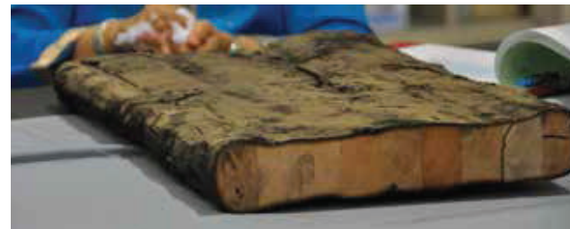
Thick timber columns like Glulam will initially ignite but the charring of the outer layers of wood will cut off the oxygen supply and effectively slows down the burning of the deeper layers of the timber.
